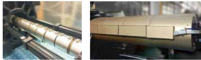
Infrared barrel heating system (optional)
